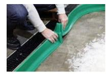
Do not let any oils or solvents enter the sewer / stormwater system. Use any available material to construct a barrier.
